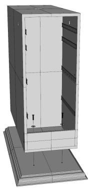
To start, remove all the drawers from the cabinets. Push the plastic tabs in each drawers guide Up on one side and Down on the other and simply slide the drawer out.
